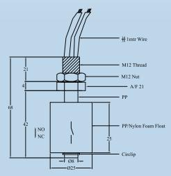
To Reverse Actuation: Remove circlip and reverse the Float
